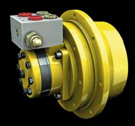
Wheel drives come in 5 sizes with a maximum torque ranging between 800 and 3,500 Nm. These models are suitable for track drive and wheel drive applications due to the relatively high load supported by the bearings (8,000 kg in the EH models). Several accessories are available (including static brake, disengagement system, and control valves).
